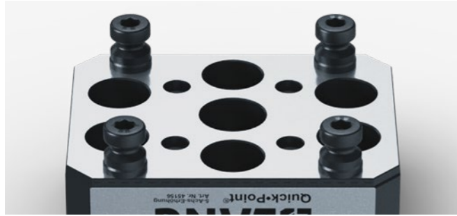
The Quick-Point® 52 Riser also features bores for Ø 20 mm clamping studs in order to being able to use it as an adaptor for the 96 mm grid system.
